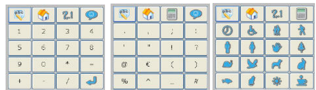
Figure 3. The three-fold layout of the miscellaneous keypad according to the selected mode (left: number selection, middle: punctuation, right: pre-recorded messages)
